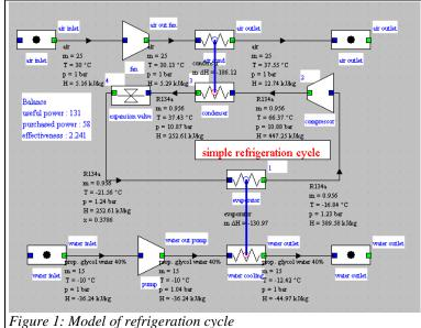
somewhat the model we assume that the value of the evaporation superheating remains constant (5 K). The condensation sub-cooling, however, is determined on the basis of the overall mass of refrigerant, which remains constant in the machine.
