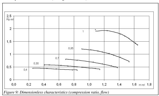
The mass flow rate depends on the thermodynamic state at the suction and compression ratio.
