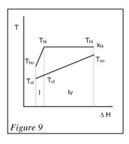
$$\epsilon_l \ = \frac{T_{hi} \ \text{-} \ T_{ho}}{T_{hi} \ \text{-} \ T_{ci}} \qquad \qquad R_l = \frac{m_h C p_{hl}}{m_c C p_c} \label{eq:epsilon}$$
