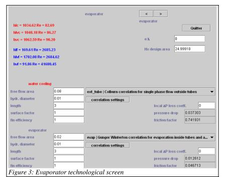
of 2 dm 2 and a hydraulic diameter of 1 cm, the tubing length being 3 m. Choose the type of configuration ("evap Gungor Winterton" for evaporation inside the tubes for the "evaporator" (refrigerant), and "ext tube Colburn correlation" for the brine, and set the screen as shown Figure 3.
