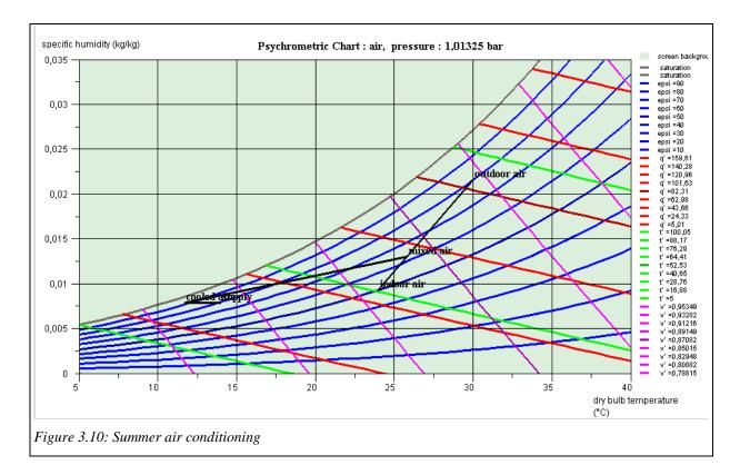
The air processing cycle is shown in the chart, the mixed air being as required on the mixing line that connects the inside air and outside air.
