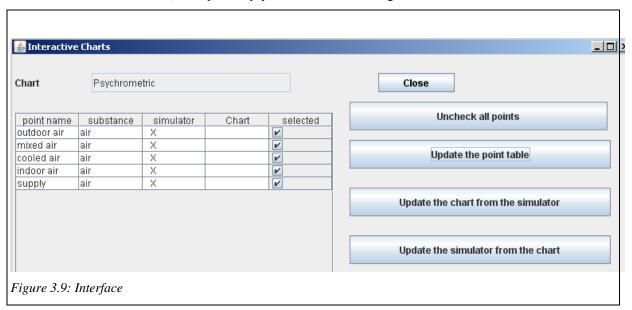
Update the table of points, then the chart from the simulator. Finally, select "Points connected" in the menu "Cycle". The cycle plot on the psychrometric chart is given in Figure 3.10.
