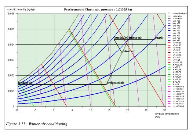
The problem data are as follows: we seek to maintain the atmosphere inside the building at a temperature of 20 °C and a relative humidity of 30%. External climatic conditions are: temperature equal to -10 °C and relative humidity of 90%. We must provide a heat input of 100 kW off ventilation, but no water. To avoid parasite condensation, fresh air is preheated at 14 °C (point 1).
